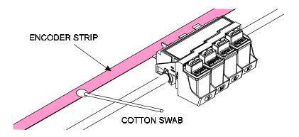
Figure 3-1. Encoder Strip Cleaning.
